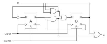
(ii) (3 points) Derive the Boolean equations for the inputs of the flip-flops (DA, DB) and the output (Z).
