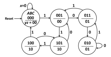
(iii) (4 points) Using K-maps, obtain the minimized next-state equation at the input of flip flop C and for the output y. For the unused states, assume that they always make a transition to the start state, regardless of the input x. The output of all unused states should be yz = 11.
