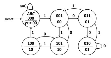
(i) (5 points) Complete the timing diagram for the above state diagram, showing the waveforms of the state variables A, B, C, and the outputs y and z. Initially, the flip-flops are reset to 0.
