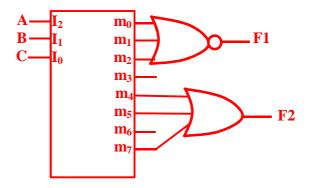
e. Convert the circuit below to **2-input NAND gates only.** Redraw the circuit to obtain a multi-level NAND circuit implementation. Assume that **both the true and complement** forms of each input variable are available. **Use the circuit as is and do not attempt to simplify it.** (5 Marks)
