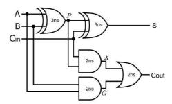
a) Write **a gate-level** Verilog description of the above full adder using the Inputs, Outputs, and wire names and gate delays shown on the diagram above. (5 Marks)
