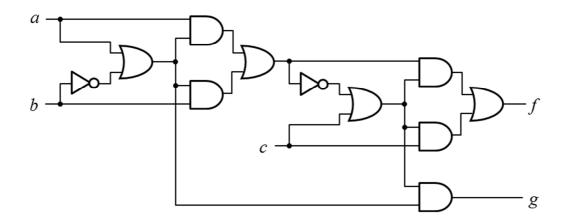
Redraw the above circuit diagram **using only NAND gates** and a minimum number of inverters (NOT gates). You may insert inverters only when necessary.
