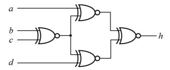
Redraw the above circuit **using only XOR gates** and a minimal number of inverters. You may insert inverters only when necessary.
