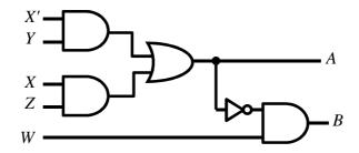
a) Write a Verilog module (call it **CC**) describing this circuit, *as is*, using primitive gates. Assume the following gate delays; inverter's delay= 1 (time unit), AND's delay= 2, OR's delay=3. **[5 marks]**
