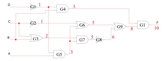
The propagation delay of F = 10ns The critical path of F is G1 - G5 - G7 - G8 - G9 - G10
