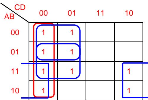
PIs (both blue and red):  $A\bar{D}, \bar{A}\bar{C}, B\bar{C}, \bar{C}\bar{D}$
