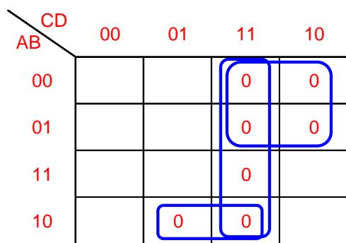
$$F(A, B, C, D) = POS = (\bar{A} + B + \bar{D}) \cdot (\bar{C} + \bar{D}) \cdot (A + \bar{C})$$
