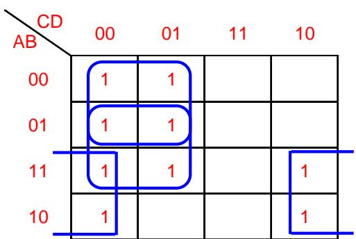
$$F(A, B, C, D) = SOP = A\bar{D} + \bar{A}\bar{C} + B\bar{C}$$
