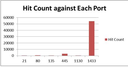
Figure 3. Analysis of the hit counts against the open TCP ports
