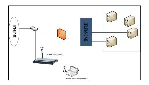
Figure 7: The ADSL deployment scenario for the pilot run
