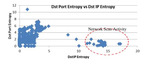
Figure 21: Destination Port entropy and Destination IP entropy combination of SSH Honeypot trace
