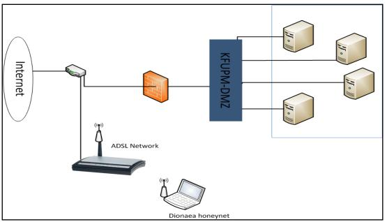
Figure 2. The ADSL deployment scenario for the pilot run
