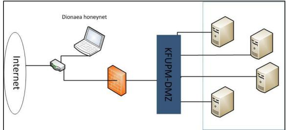
Figure 1. The Pilot deployment map on the KFUPM network
