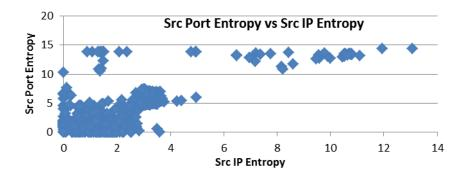
Figure 22: Source IP entropy and Source Port entropy combination of SSH Honeypot trace
