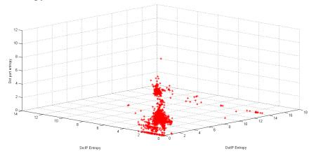
Figure 23: Combination of Destination port, Source IP and Destination IP Entropy values
