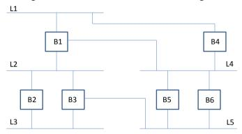
Suppose fixed routing is used to configure the bridges. Determine the central routing directory for all segments, and the routing tables for Bridges B3 and B5. If alternate routes are available then chose the one with the least number of hops. If they are the same than choose the one with the lowest bridge ID.
