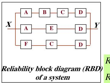
The above equation is an upper bound because the paths are not independent. That is, the failure of a single module affects more than one path.
