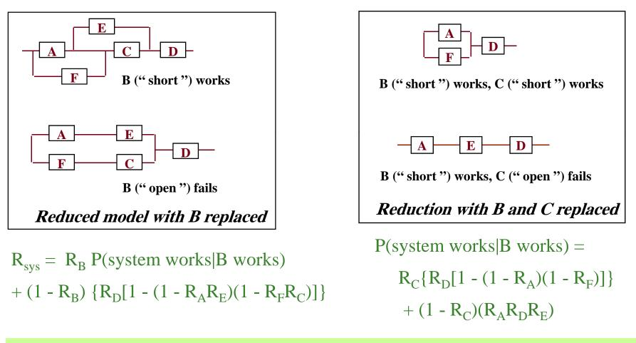
Letting  $R_A = \ldots = R_F = R_m$  yields  $R_{sys} = R_m^6 - 3R_m^5 + R_m^4 + 2R_m^3$
