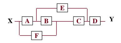
Each path from X to Y represents a configuration that leaves the system successfully operational
