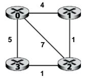
Suppose that the link cost c(0,3) has changed from 5 to 1, re-compute the distance tables for nodes 0, 1, 2, and 3 after <u>only one</u> iteration of a synchronous version of the distance vector. Note that the current tables' values <u>prior</u> to the link cost change are as shown in the leftmost column of the tables.
