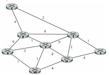
With the indicated link costs, use Dijkstra's shortest-path algorithm, as discussed in class, to compute the shortest path from t to all network nodes using the table given below.
