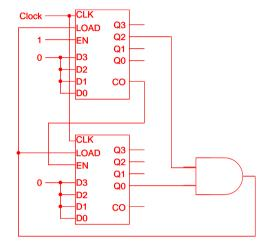
Note that the counter uses 5 bits  $b_4b_3b_2b_1b_0$  to be able to count from 0 to 20. The counter at the top of the diagram will represent  $b_3$ ,  $b_2$ ,  $b_1$ , and  $b_0$ , using Q3, Q2, Q1, and Q0, respectively. On the other hand, the counter at the bottom of the diagram will represent  $b_4$  using Q0.
