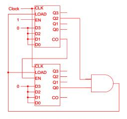
Note the counter uses 5 bits  $b_4b_3b_2b_1b_0$  to be able to count from 0 to 20. The counter at the top of the diagram will represent  $b_3$ ,  $b_2$ ,  $b_1$ , and  $b_0$ , using Q3, Q2, Q1, and Q0, respectively. On the other hand, the counter at the bottom of the diagram will represent  $b_4$  using Q0.
