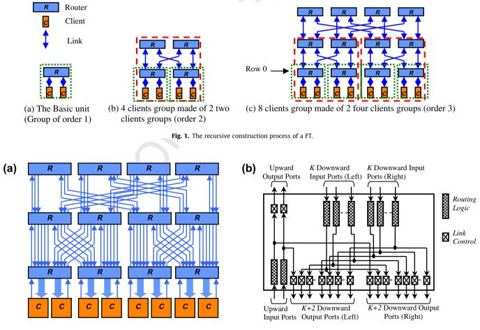
Fig. 2. (a) The original MFT topology and (b) router architecture with downward link doubling (geometrical link progression).
