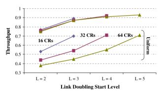
Fig. 14. Throughput versus link doubling start level for the controlled geometrical link progression scheme for three NoC sizes and for uniform (bottom group of curves) and non-uniform traffic.
