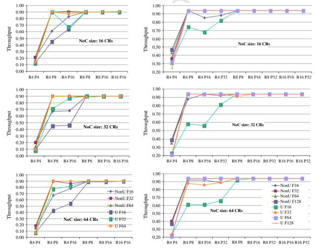
**Fig. 11.** Measured throughput versus FIFO emptying rate (*R*) and parallelizer's width (*P*) for 3 NoC sizes, several FIFO sizes, uniform and non-uniform traffic models. Results on the left are for a packet size of 32 bytes while results on the right are for a packet size of 64 bytes.
