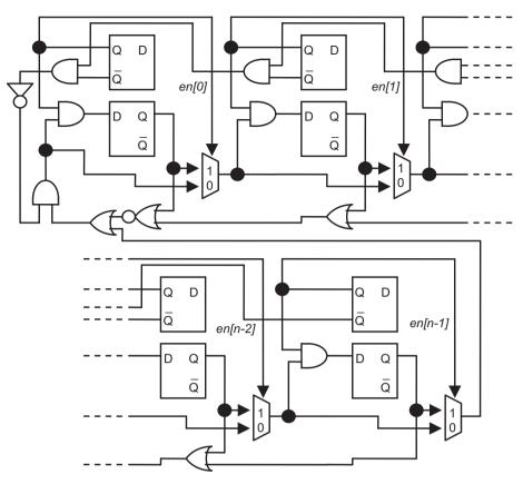
Fig. 6. Schematic of the request propagation circuit at the heart of the intelligent polling scheme.
