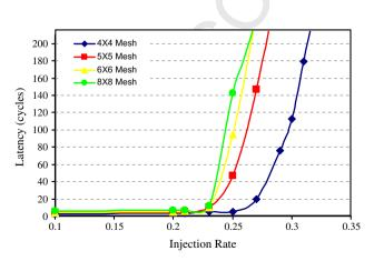
Fig. 16. Average latency versus injection rate for mesh-based network of various sizes.
