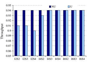
**Fig. 13.** Throughput as a function of link progression parameters (increment *I* and stop level *S*) for arithmetic progression (left) and mixed arithmetic/geometrical progression (right) for uniform (U) and non-uniform (NU) traffic.
