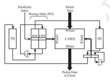
Fig. 7. The structure of the central FIFO.
