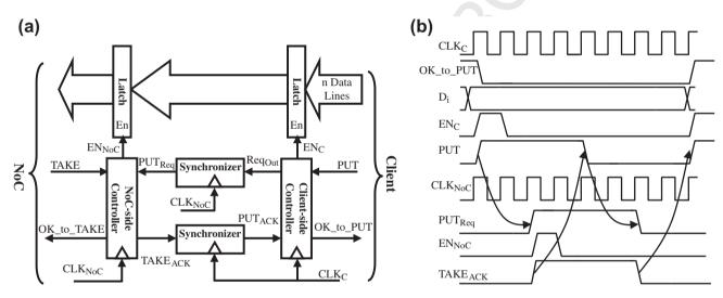
Fig. 8. The proposed circuitry for data transfer between two clock domains; (a) the basic block diagram, (b) the signaling protocol for equal clock frequencies.
