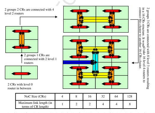
Fig. 3. The H-tree construction of the NoC floor plan (not to scale). The client/NoC interface (CNI) is at the edge of the NoC at the client's interface to the 1st level of routers (row 0).
