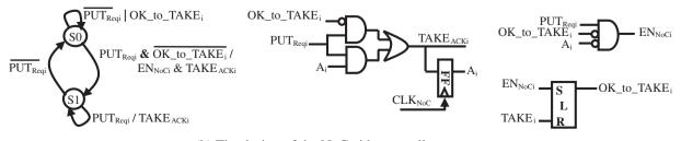
(b) The design of the NoC-side controller.
