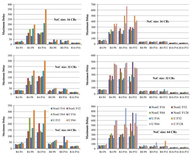
**Fig. 12.** Measured maximum packet delay versus FIFO emptying rate (*R*) and parallelizer's width (*P*) for 3 NoC sizes, several FIFO sizes, uniform and non-uniform traffic models. Results on the left are for a packet size of 32 bytes while results on the right are for a packet size of 64 bytes.
