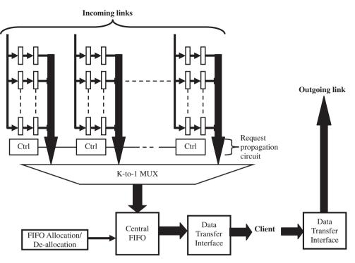
Fig. 5. Block diagram of the client network interface (CNI).
