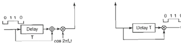
Figure 3.11 Differentially encoded BPSK.
