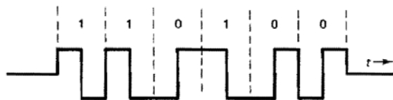
Figure 2.9 Manchester coding. A binary 1 is mapped into a positive pulse followed by a negative pulse, and a binary 0 is mapped into a negative pulse followed by a positive pulse. Note the transition in the middle of each signal interval.
