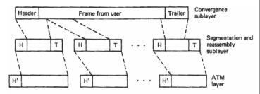
Figure 2.57 Headers and trailers at the convergence sublayer and segmentation and reassembly sublayer of the adaptation layer. Note that the user frame and its convergence sublayer header and trailer need not completely fill the data area at the segmentation and reassembly sublayer. The data plus header and trailer at the segmentation and reassembly sublayer must be exactly 48 bytes in length, however, to fit into the ATM data area.
