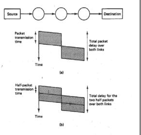
Figure 2.37 Decreasing delay by shortening packets to take advantage of pipelining.
