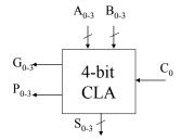
Accepts two 4-bit numbers A and B with initial carry signal  $C_0$  Generates 4-bit summation in addition to group generate/functions To do 4-bit additions – one needs to add logic to generate  $C_4$  signal using  $C_{0-3}$ ,  $C_{0-3}$ , and  $C_0$
