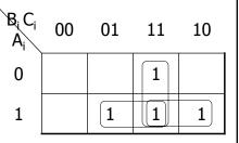
$$S_{i} = \overline{A_{i}} \overline{B_{i}} C_{i} + \overline{A_{i}} \overline{B_{i}} \overline{C_{i}} + A_{i} \overline{B_{i}} \overline{C_{i}} + A_{i} B_{i} C_{i} \qquad C_{i+1} = A_{i} B_{i} + A_{i} C_{i} + B_{i} C_{i}$$
