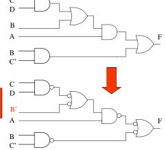
Note: an inverter is added to the path for the literal B
