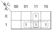
$$S_{i} = \overline{A_{i}} \overline{B_{i}} C_{i} + \overline{A_{i}} B_{i} \overline{C_{i}} + A_{i} \overline{B_{i}} \overline{C_{i}} + A_{i} B_{i} C_{i}$$
