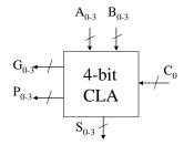
Accepts two 4-bit numbers A and B with initial carry signal  $C_0$  Generates 4-bit summation in addition to group generate/functions To do 4-bit additions – one needs to add logic to generate  $C_4$  signal using  $G_{0-3}$ ,  $P_{0-3}$ , and  $C_0$
