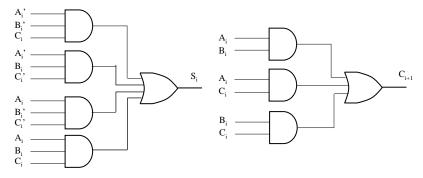
$\tau$  is the logic gate delay (including the inverter)  $S_i$  output is available after  $3\tau$  delay
