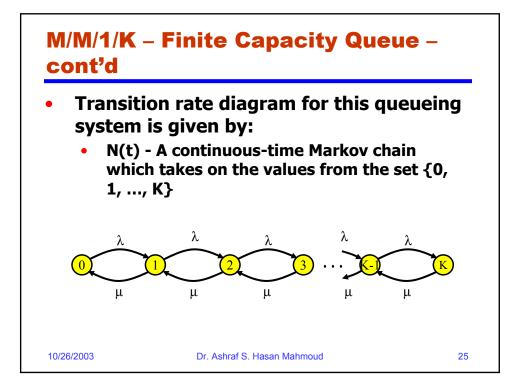
M/M/1/K – Finite Capacity Queue – cont'd The global balance equations:  $\mathbf{p}_0 = \mu \mathbf{p}_1$ λ  $(\lambda + \mu)p_j = \lambda p_{j-1} + \mu p_{j+1}$  for j=1, 2, ..., K-1  $\mathbf{p}_{\kappa} = \lambda \mathbf{p}_{\kappa-1}$ μ  $\rightarrow$  Prob[N(t) = j] = p<sub>j</sub> **j=0,1, ..., K;** ρ<**1**  $= (1-\rho)\rho^{j}/(1-\rho^{K+1})$ When  $\rho = 1$ ,  $p_i = 1/(K+1)$  (all states are equiprobable) 10/26/2003 Dr. Ashraf S. Hasan Mahmoud 26
