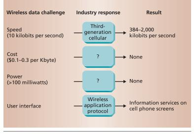
Figure 2. To implement wireless data technology, two complementary approaches have been developed: 3G, a third-generation cellular radio transmission technology, and WAP, the wireless application protocol.
