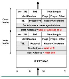
Home agent encapsulated the IP Packet inside an other IP header and Sends it to the care-of-address of mobile
