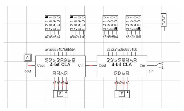
h. Determine by simulation the longest delay in the 8-bit adder in (g).
