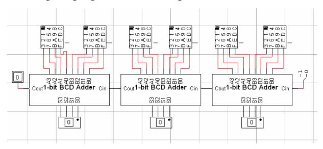
c. Verify the correct functionality of the 3-digit BCD adder by simulating the following operations: 999 + 1, 999+222, 100+999, 279+465
