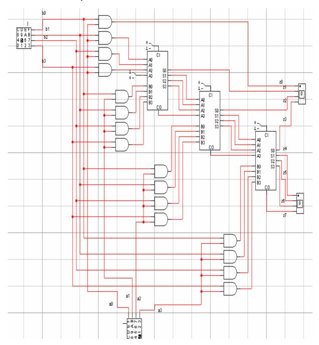
b. Verify the correct functionality of the 4-digit multiplier by simulating the following operations: 15\*1, 15\*0, 5\*5, 2\*8, 8\*7, 15\*15.
