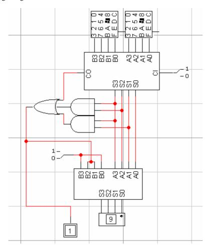
b. Using the single digit BCD adder, build a 3-digit BCD adder.
