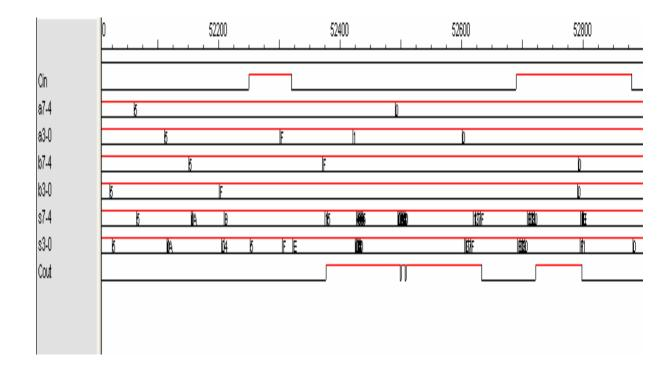
c. Determine the worst case delay in your 8-bit Ripple Carry Adder by simulation.
