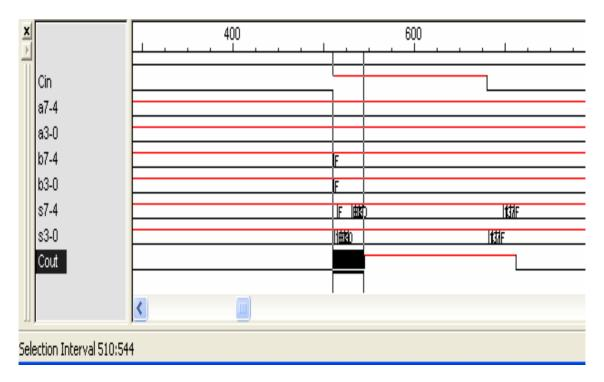
As can be seen, the delay from the Cin signal to the Cout signal is 544-510= 34ns.
