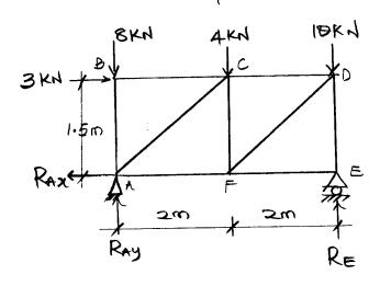
External reactions  $2M_{A} = 4R_{E} - 3(1.5) - 4(2) - 10(4) = 0$   $4R_{E} = 52.5$   $R_{E} = \frac{52.5}{4} = 13.125 \text{ KA}$   $2F_{A} = R_{A} - 3 = 0$  $R_{A} = 3 \text{ KA}$
