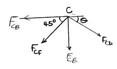
$$\Sigma F_{y} = -F_{cF} \sin 45^{\circ} - F_{cE} - F_{cD} \sin 0 = 0$$
