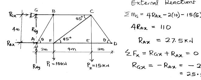
External Reactions ZMG = 4RAX-2(10)-15(6) =0  $R_{GX} = -R_{AX} = -27.5 \text{ kd}$
