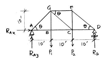
External Reactions  $\frac{2M+ = 30R_0 - 10(500) - 20(1500) = 0}{R_0 = 1166.66716}$ No horizontal loading, so RAX = 0
