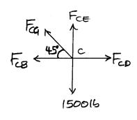
$$2F_{x} = -F_{c8} - F_{ca}C_{5}45^{\circ} + F_{cb} = 0$$
