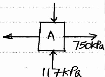
Note that the internal pressure due to water does not cause longitudinal stress in the open tank. (why?!)
