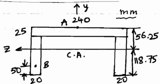
To calculate  $\sigma$  and  $\tau$ , we need to determine the internal forces at a section 2-m from left that passes through A and B, as shown in the FBD below.
