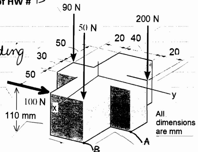
First, we need to determine the internal forces at the bottom of the block (through A and B), as shown (FBD).
