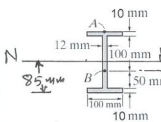
$$I_{NA} = \frac{100 \times 170^3}{12} - \frac{88 \times 150^3}{12} = 1.619 \times 10^7 \text{ mm}^4$$
