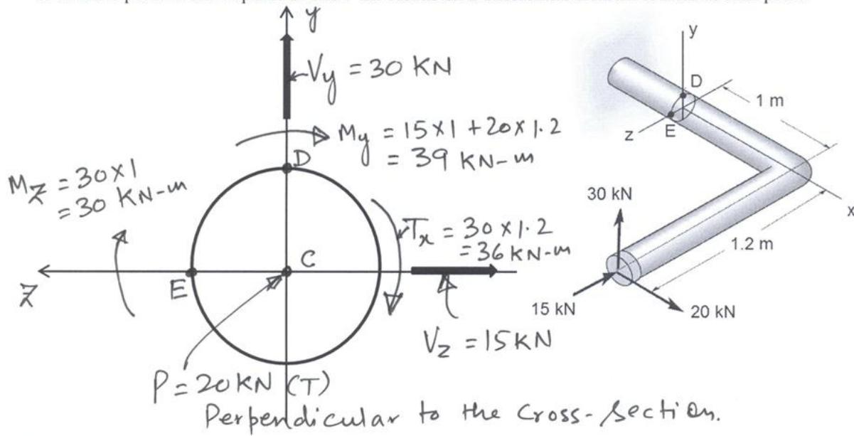
$$\sigma_D = \frac{P}{A} - \frac{M_Z \times y}{I} = \frac{20 \times 10^3}{\pi \times 30^2} - \frac{30 \times 10^6 \times 30}{\frac{\pi}{4} \times 30^4} = 7.07 - 1414.71 \\ = -1407.64 \text{ N/mm}^2 = 1407.64 \text{ N/mm}^2 (\text{Comp.})$$
