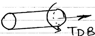
$$\tau_{max} = \frac{T_{AB} r_{max}}{J} = \frac{20(10)(10)^{-3}}{\pi/2 [ (10)(10)^{-3} ]^4} = 12.732 \text{ MPa.}$$
