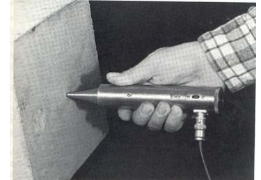
Exponential probe transducers used for UPV test on rough or curved surfaces
