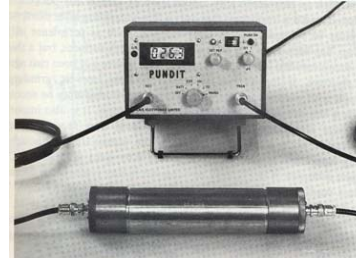
PUNDIT Equipment with flat transducers popularly used for UPV test
