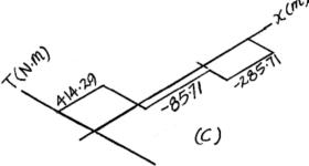
5–90. The two 3-ft-long shafts are made of 2014-T6 aluminum. Each has a diameter of 1.5 in. and they are connected using the gears fixed to their ends. Their other ends are attached to fixed supports at A and B. They are also supported by bearings at C and D, which allow free rotation of the shafts along their axes. If a torque of 600 lb·ft is applied to the top gear as shown, determine the maximum shear stress in each shaft.
