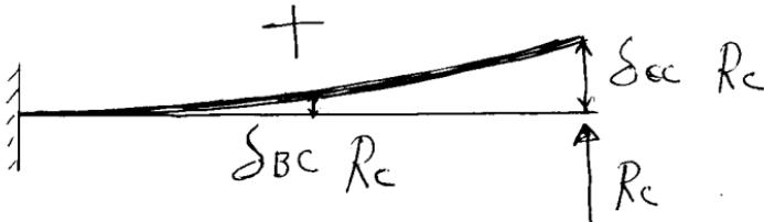
$$\left\{ \begin{matrix} \Delta_B \\ \Delta_C \end{matrix} \right\} + \left[ \begin{matrix} \delta_{BB} & \delta_{BC} \\ \delta_{CB} & \delta_{CC} \end{matrix} \right] \left\{ \begin{matrix} R_B \\ R_C \end{matrix} \right\} = \left\{ \begin{matrix} 0 \\ \frac{R_C(10)}{0.01 \times 10000} \end{matrix} \right\}$$
