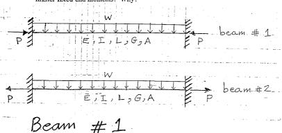
(b) The two beams shown are identical in everything except the moment of inertia. Which beam will have higher reactions? Why?
