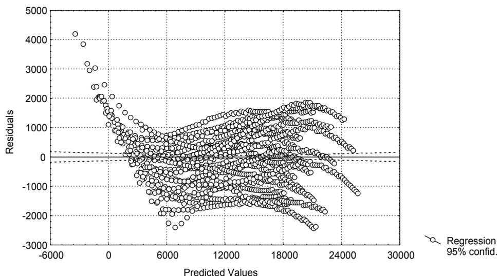
Figure 4: Predicted versus residuals of estimation for the prediction of the absolute maximum stresses for the pipe constructed on low density sand
