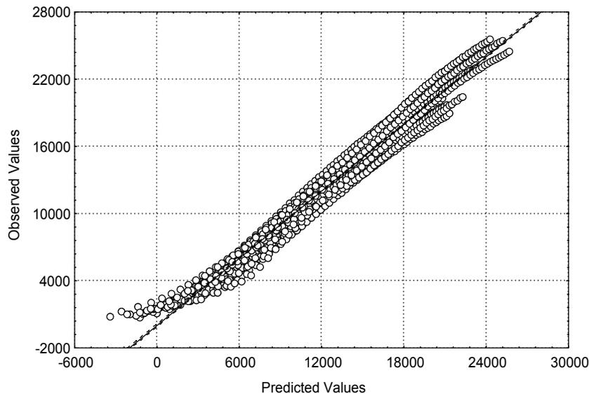
Figure 3: Plot of predicted versus calculated absolute maximum stresses for the pipe constructed on low density sand.
