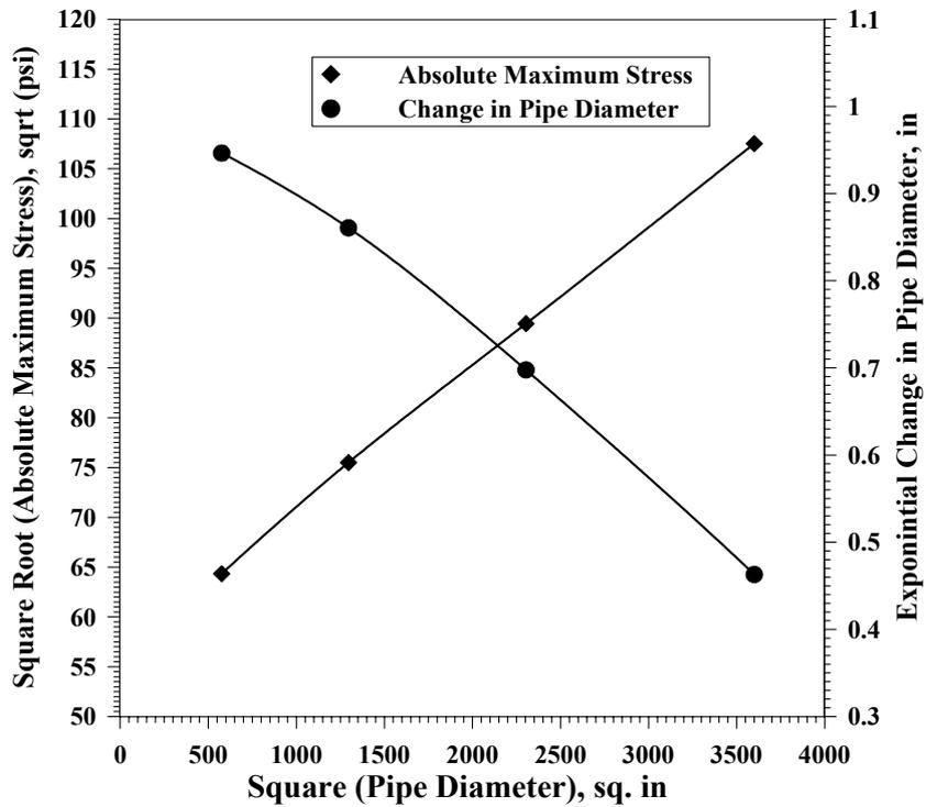
Figure 2: Linearization of the pipe diameter and absolute maximum stress and change in pipe diameter relationship.
