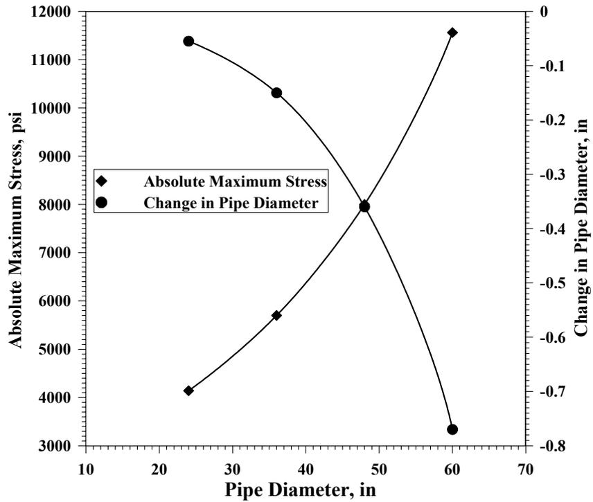
Figure 1: Relationship between pipe diameter and both absolute maximum stress and change in pipe diameter.
