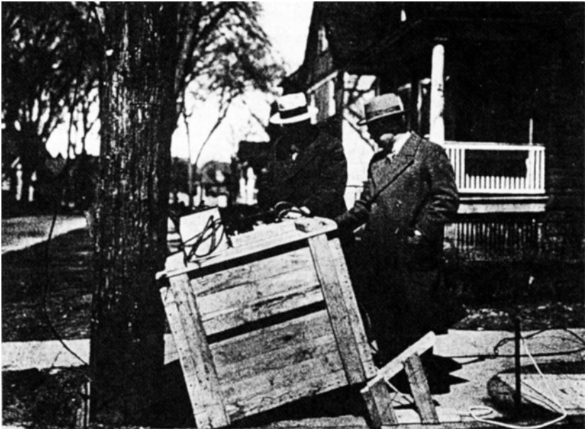
FIGURE 3. Earlier use of X-ray diagnosis techniques for imaging the inner condition of the trunk of a street tree. From (Maloy and Wilsey, 1930).
