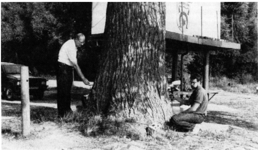
FIGURE 1. Description of the Stress Wave Timer technique. Top: principle (Bethge et al. , 1996), and bottom: in practice (Mattheck and Bethge, 1992).
