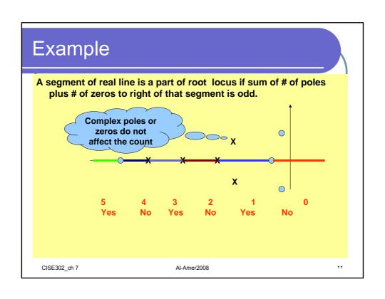
+ Step 2: Segments of real axis that are parts of the root locus
