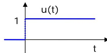
Figure 3.1 Unit Step Function
