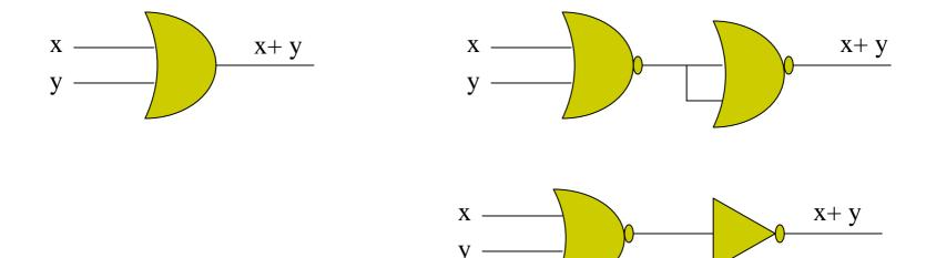
OR operation can be implemented using NOR gates
