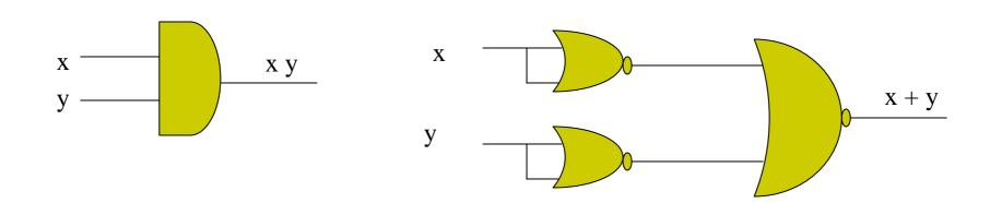
AND operation can be implemented using NOR gates
