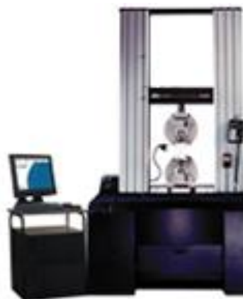
Tensile testing machine for metals and polymers
