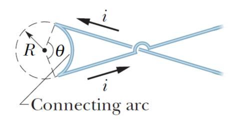
The outward field (the field of the two semi-infinite wires) is equal to the field of the arc but opposite to it. Thus,
