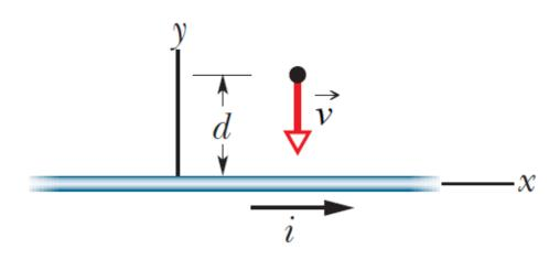
tion, what is the magnetic force on the proton due to the current?
