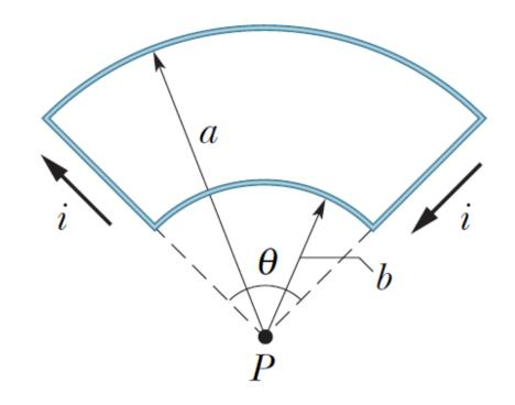
a) The field due to the straight segments at point *P* is zero. The right hand rule tells us that the magnetic field due the small and large arcs at point *P* are out of the page and into the page, respectively.
