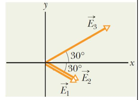
The net electric field  $\vec{E}=\vec{E}_3+\vec{E}_{12}$  is in the positive x direction. Its magnitude is
