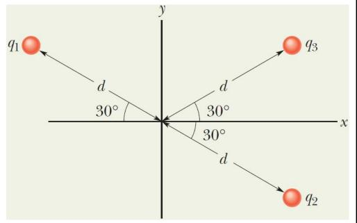
$\vec{E}_1$  and  $\vec{E}_2$  are in the same direction. Their resultant electric field  $\vec{E}_{12}$  has the same direction and has the magnitude
