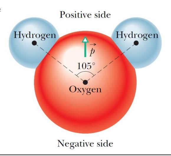
**Example 4**: A neutral water molecule (H<sub>2</sub>O) in its vapor state has an electric dipole moment of magnitude  $6.2 \times 10^{-30}$  C·m.
