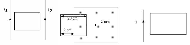
4- The square coil shown in the figure is 20 cm on a side and has 15 turns of wire on it. It is moving to the right at 2 m/s. Find the induced emf in it at the instant shown, and the direction of the induced current in the coil. (The magnetic field is 0.2 T and its direction is out of the page). [1.2 V, clockwise]
