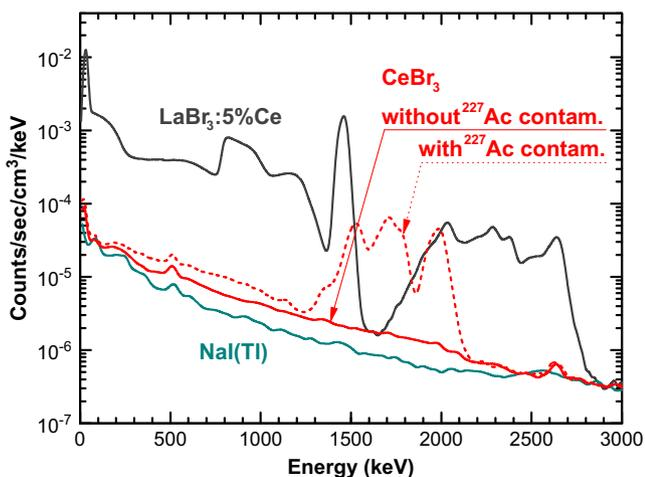
Fig. 8. Intrinsic activity spectrum of CeBr<sub>3</sub>, LaBr<sub>3</sub>:5%Ce and NaI(Tl) 2" × 2" spectrometers. For CeBr<sub>3</sub> two spectra are reported corresponding to crystal with and without <sup>227</sup>Ac contamination.
