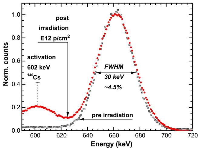
Fig. 12. Close-up of  $^{137}\text{Cs}$  pulse height spectra collected with  $\text{CeBr}_3$   $1'' \times 1''$  sample SFC 273 (Tables 1 and 2) pre-irradiation and 16 days after irradiation with  $10^{12}$  protons/cm $^2$ .
