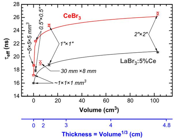
**Fig. 3.** Scintillation decay time under <sup>137</sup>Cs excitation for both CeBr<sub>3</sub> and LaBr<sub>3</sub>:5% Ce samples of several volumes. The two lines are interpolating logarithmic functions to guide the eyes. The 30 mm × 8 mm CeBr<sub>3</sub> sample represents a deviant data point (open diamond data symbol) which is attributed to its particular aspect ratio.
