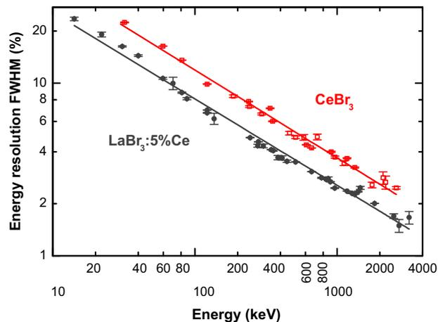
Fig. 7. Energy resolution FWHM as function of photon energy for  $2'' \times 2''$  spectrometer based on  $\text{CeBr}_3$  and  $\text{LaBr}_3:5\%\text{Ce}$ . The lines are the best fitting function of Eq. (2).
