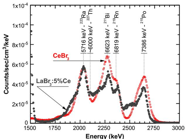
Fig. 10.  $\text{CeBr}_3$  and  $\text{LaBr}_3:5\%\text{Ce}$  intrinsic activity spectra of Fig. 8 ( $2'' \times 2''$  samples) using a common energy calibration, i.e. that of  $\text{LaBr}_3:5\%\text{Ce}$ . The 5 alpha peaks are labeled according to [28,31].
