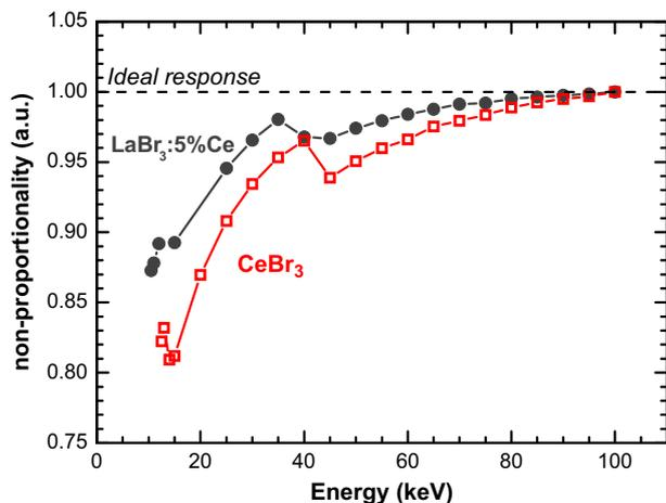
Fig. 4. Synchrotron measurements of the non-proportionality of the response (nPR) of CeBr<sub>3</sub> and LaBr<sub>3</sub>:5%Ce. The curves are normalized to 1 at 100 keV.
