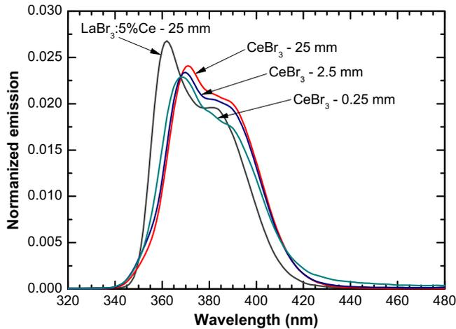
**Fig. 2.** X-ray excited emission of CeBr<sub>3</sub> and LaBr<sub>3</sub>:5%Ce. For CeBr<sub>3</sub>, the emission of three samples with increasing thicknesses is presented. The spectra are area normalized.
