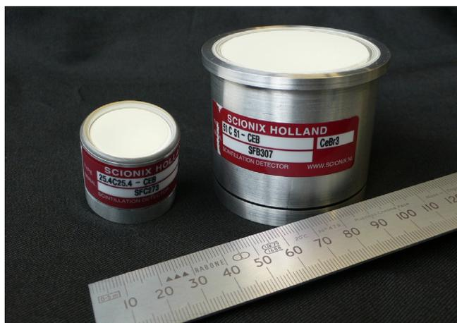
**Fig. 1.** Picture of two of the CeBr<sub>3</sub> encapsulated samples used in this study, left 1" × 1" sample SFC 273 (proton irradiated) and right 2" × 2" sample SFB 307.
