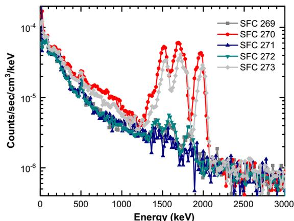
Fig. 9. Intrinsic activity spectrum of 5 CeBr<sub>3</sub> spectrometers with dimension of 1" × 1".
