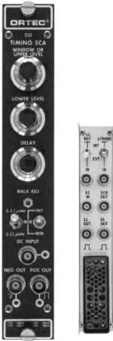
The EG&G ORTEC Model 551 Timing Single-Channel Analyzer performs the dual functions of single-channel pulse-height analysis and timing signal derivation.
