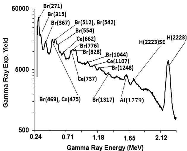
Fig. 4 Activation spectrum of the CeBr<sub>3</sub> Detector
