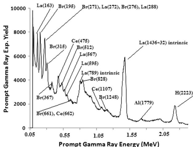
Fig. 6 Activation spectrum of LaBr<sub>3</sub>:Ce detector taken from ref. [4]
