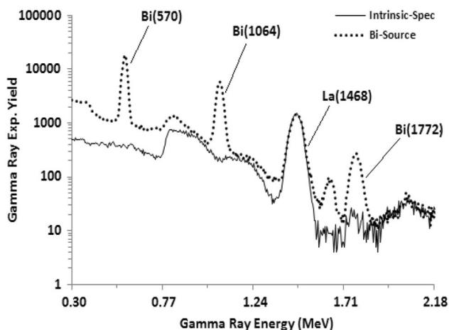
**Fig. 2**  $\text{LaCl}_3\text{:Ce}$  detector Intrinsic activity spectrum superimposed upon  $^{207}\text{Bi}$  source spectrum
