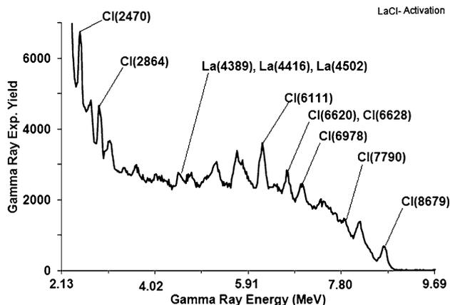
Fig. 8 Portion of Activation spectrum of LaCl<sub>3</sub>:Ce detector
