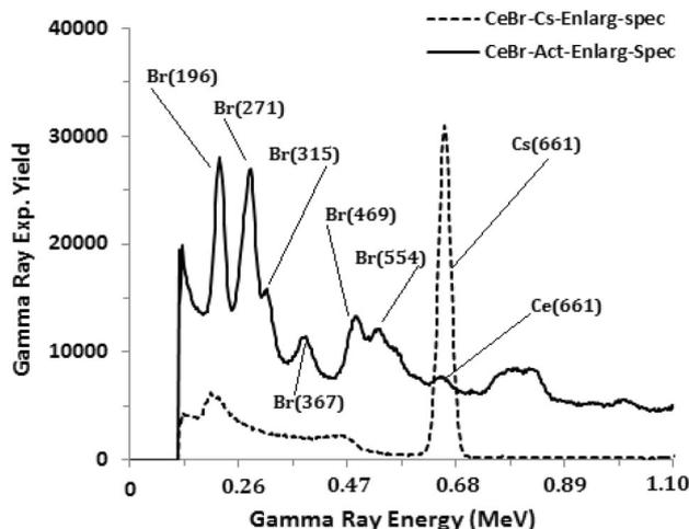
Fig. 5 Portion of CeBr<sub>3</sub> activation spectrum superimposed upon <sup>137</sup>Cs Source spectrum
