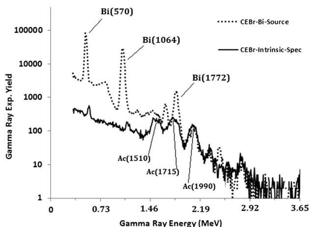
**Fig. 1** CeBr<sub>3</sub> detector intrinsic activity spectrum superimposed upon <sup>207</sup>Bi source spectrum
