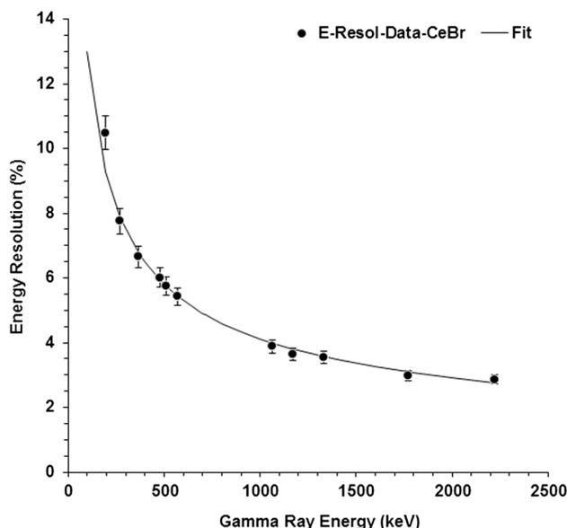
Fig. 9 Energy resolution  $\Delta E/E$  (%) data of the CeBr<sub>3</sub> detector superimposed upon least square fit of type  $\Delta E/E$  (%) =  $a/E^b$
