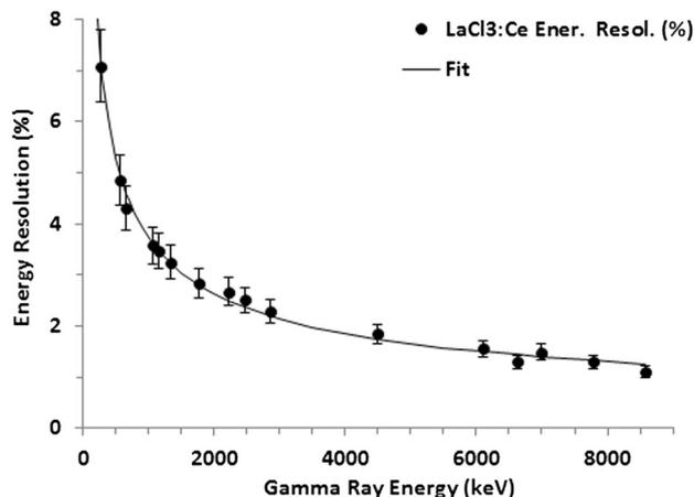
Fig. 10 Energy resolution  $\Delta E/E$  (%) data of the LaCl<sub>3</sub>:Ce detector superimposed upon least square fit of type  $\Delta E/E$  (%) =  $a/E^b$
