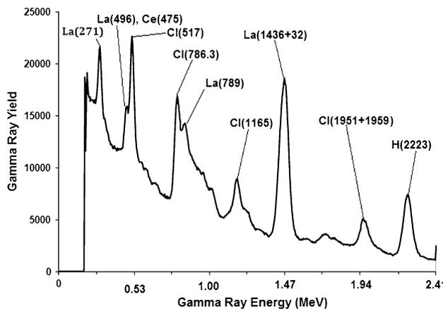
Fig. 7 Activation spectrum of LaCl<sub>3</sub>:Ce detector
