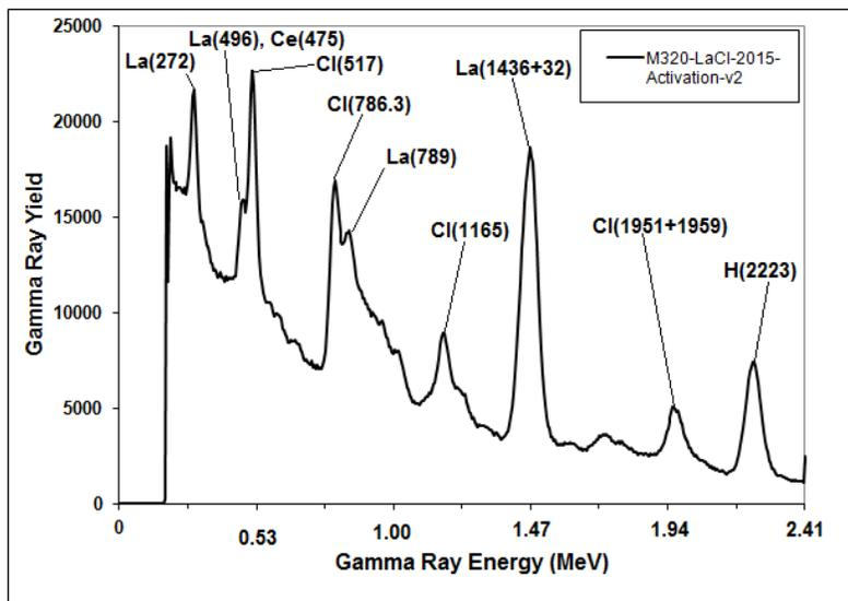
Figure 10: Low energy prompt gamma ray spectrum due to activation of  $\text{LaCl}_3:\text{Ce}$  detector caused by capture of thermal neutrons in La, Cl and Ce elements present in  $\text{LaCl}_3:\text{Ce}$  detector.
