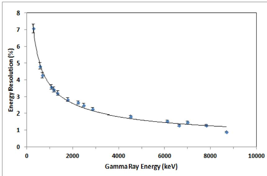
**Figure 13: Energy Resolution Curve for  $\text{LaCl}_3:\text{Ce}$  Detector with Power Fit**
