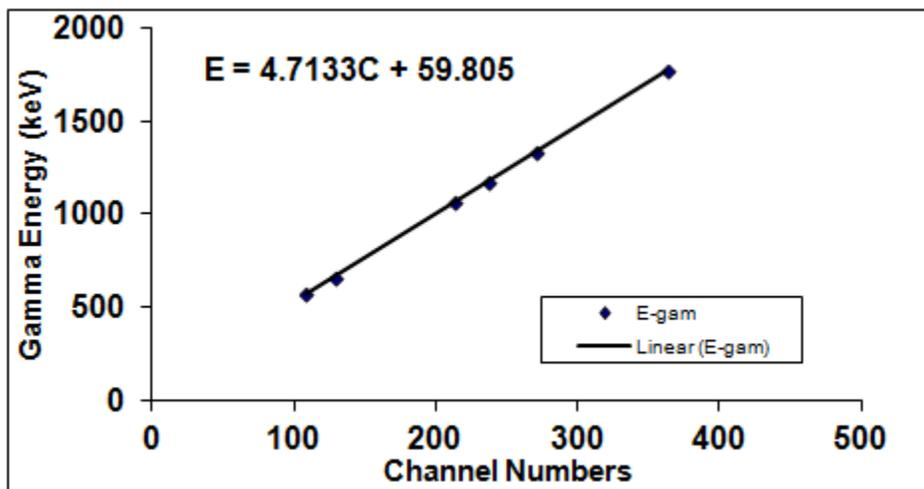
Figure 9: Low energy calibration curve of  $\text{LaCl}_3:\text{Ce}$  detector
