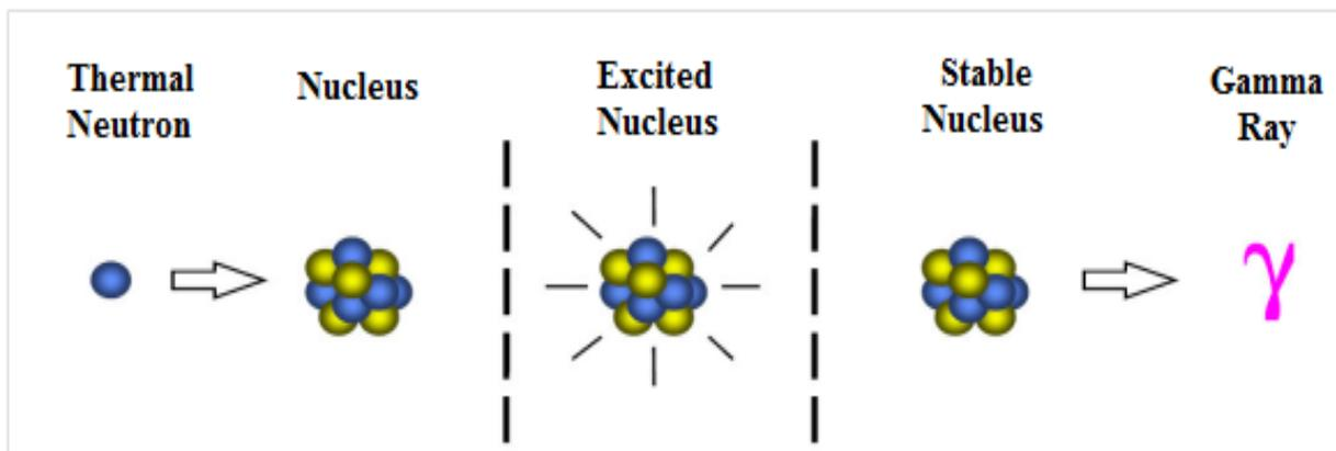
*Figure 2: Schematic diagram illustrating PGNAA process at the nucleus level.*
