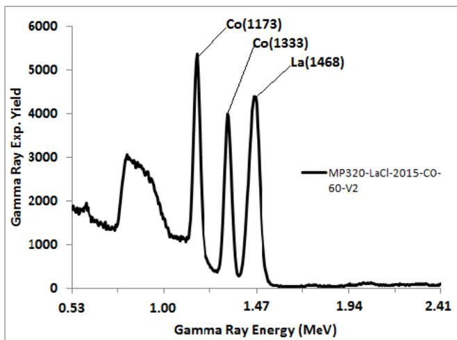
Figure 8:  $\text{LaCl}_3:\text{Ce}$  detector pulse height spectrum taken with Cobalt-60 peaks along with intrinsic peak due to La
