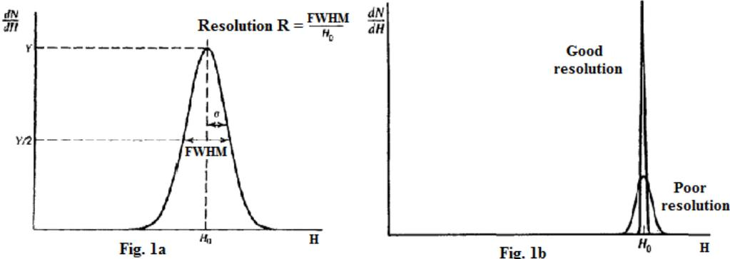
Figure 1: Shows Energy Resolution Peak and Detector Response Function
