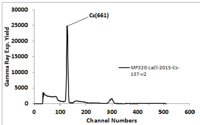
Figure 6:  $\text{LaCl}_3:\text{Ce}$  detector pulse height spectrum taken with Cesium-137 peak
