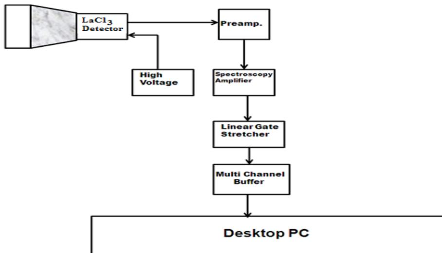
Figure 5: Electronic configuration diagram
