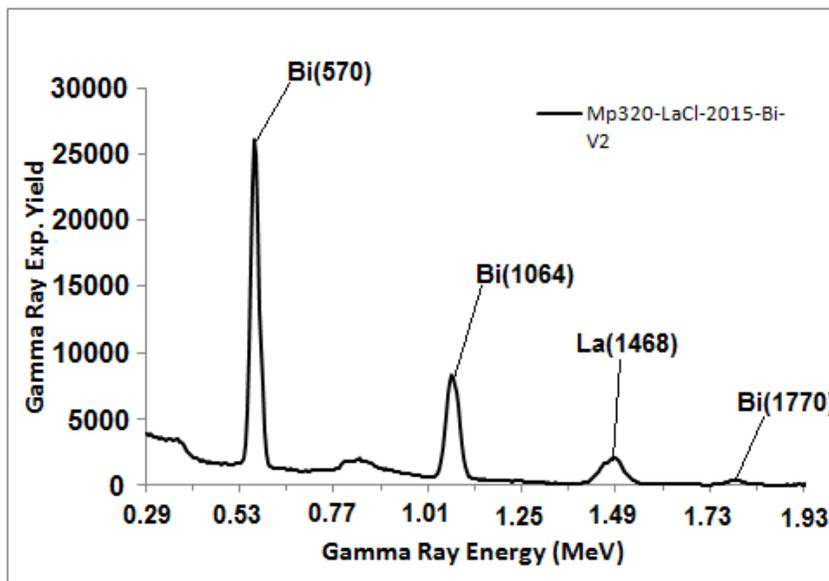
Figure 7:  $\text{LaCl}_3:\text{Ce}$  detector pulse height spectrum taken with Bismuth-209 peaks along with intrinsic peak due to La
