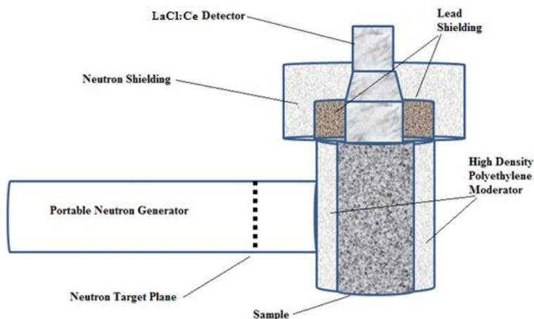
Figure 3: schematic diagram of the MP320 portable neutron generator
