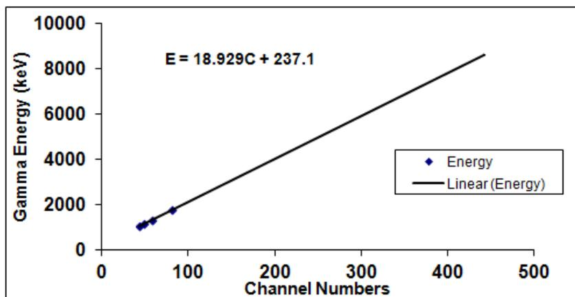
Figure 11: High energy calibration curve of  $\text{LaCl}_3:\text{Ce}$  detector
