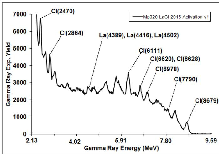
Figure 12: High energy prompt gamma ray spectrum due to activation of  $\text{LaCl}_3:\text{Ce}$  detector caused by capture of thermal neutrons in La, Cl and Ce elements present in  $\text{LaCl}_3:\text{Ce}$  detector.
