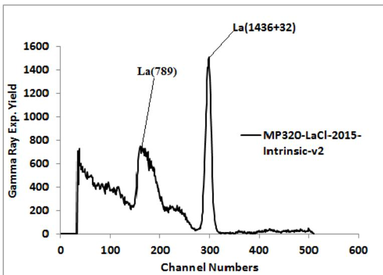
Figure 4: Intrinsic pulse height spectrum of  $LaCl_3:Ce$  detector
