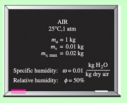
$$\phi = \frac{Mass\ of\ vapor\ in\ air}{Mass\ of\ saturated\ air} = \frac{m_v}{m_g}$$
