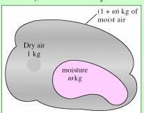
$$\omega = \frac{Mass \ of \ water \ vapor \ in \ air}{Mass \ of \ dry \ air} = \frac{m_v}{m_a}$$
