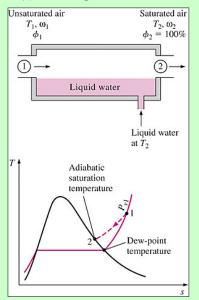
The system consists of a long insulated channel that contains a pool of water.
