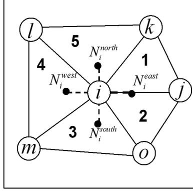
FIG. 5.2. A case where the point  $N_i^{north}$  belongs to two triangles
