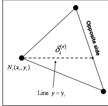
FIG. 6.2. The triangle  $\Omega_i^{(1)}$ .
