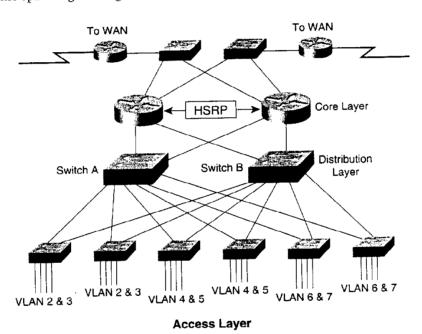
The IEEE 802.1d specification states that when multiple bridges (or switches) exist in a spanning tree, one bridge becomes the *root bridge*. Traffic always travels toward the root bridge. Only one path to the root bridge is active; other paths are disabled.
