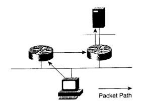
In 1989, Apple Computer, Inc., introduced AppleTalk Phase 2, which includes the best router forwarding algorithm. With the best router forwarding algorithm, a workstation can maintain a cache of the best routers to use to reach remote networks. If a destination network is in the cache, the workstation can avoid the extra-hop problem.
