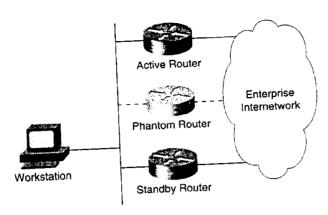
hello timer should be configured to be short enough so that workstation applications and protocols do not drop connections before the standby router becomes active.
