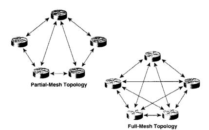
Figure 5–3 A partialmesh (left) and full-mesh (right) network topology.
