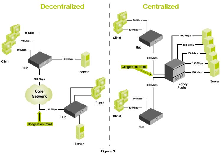
When decentralized server groups are used to optimize client traffic, bottlenecks occur between servers because the core connection becomes improperly over-subscribed. When optimizing traffic between centralized servers, client-to-server connections will suffer due to the performance limitations of legacy routers.
