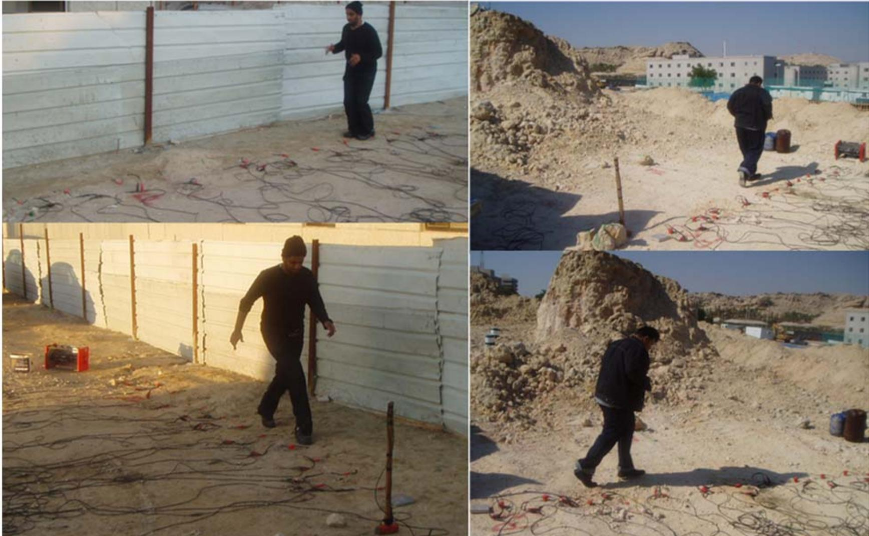
Here is what students are applying several actions as walking, running and jumping to generate adequate energy for a record of ground motion, which is required for REFRACTION MICROTREMOR (REMI).
