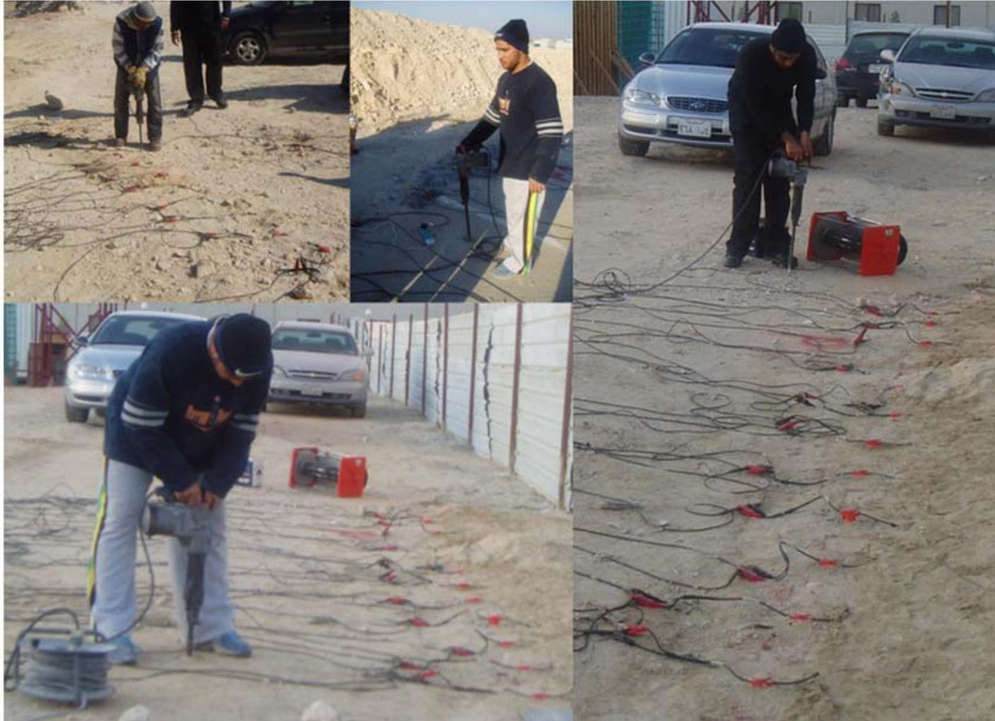
Students are trying to generate noise for 1D estimate of S-wave which is based on the records of ground waves. In general, they apply several activities of walking, jogging and hitting for making noise. Then, vibrator is used as a final solution if others do not work.
