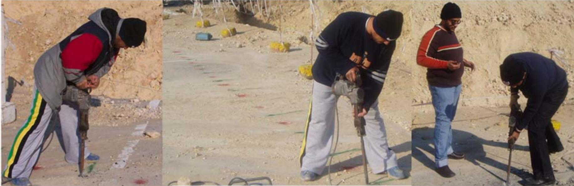
Seismic survey is required somewhere to use digging by vibrator through the hard-ground such as the asphalted areas. Thus, vibrator is also important instrument. On the other hand, it is useful to generate continuous noise. The pictures above indicate how hard digging a hole through the hard area even using a vibrator.
