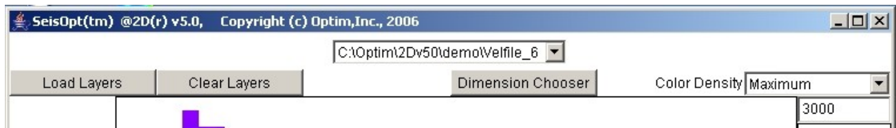
Figure 26b: Click on 'Load Layers' button on the Velfile display panel to load the 'layer_elev' file created by the 'DetLayer' module. This will plot the layers on the velocity model. Use the 'Clear Layers' button to remove the plotted layers.
