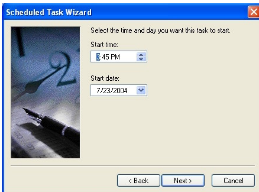
Figure 12: Set the time and date for the batch processing to start. The default setting is for the job to start immediately. Change this to be at least 10 minutes after the displayed time. If you wish to start the job immediately, click on the 'Run' option in Figure 14.
