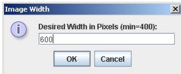
Figure 26f: Enter width of the output JPEG image in pixels. To maintain the aspect ratio of the displayed image, the ratio between the height and width (in pixels) should be similar to the numbers above the amplitude scale bar of the 'Velfile' display.
